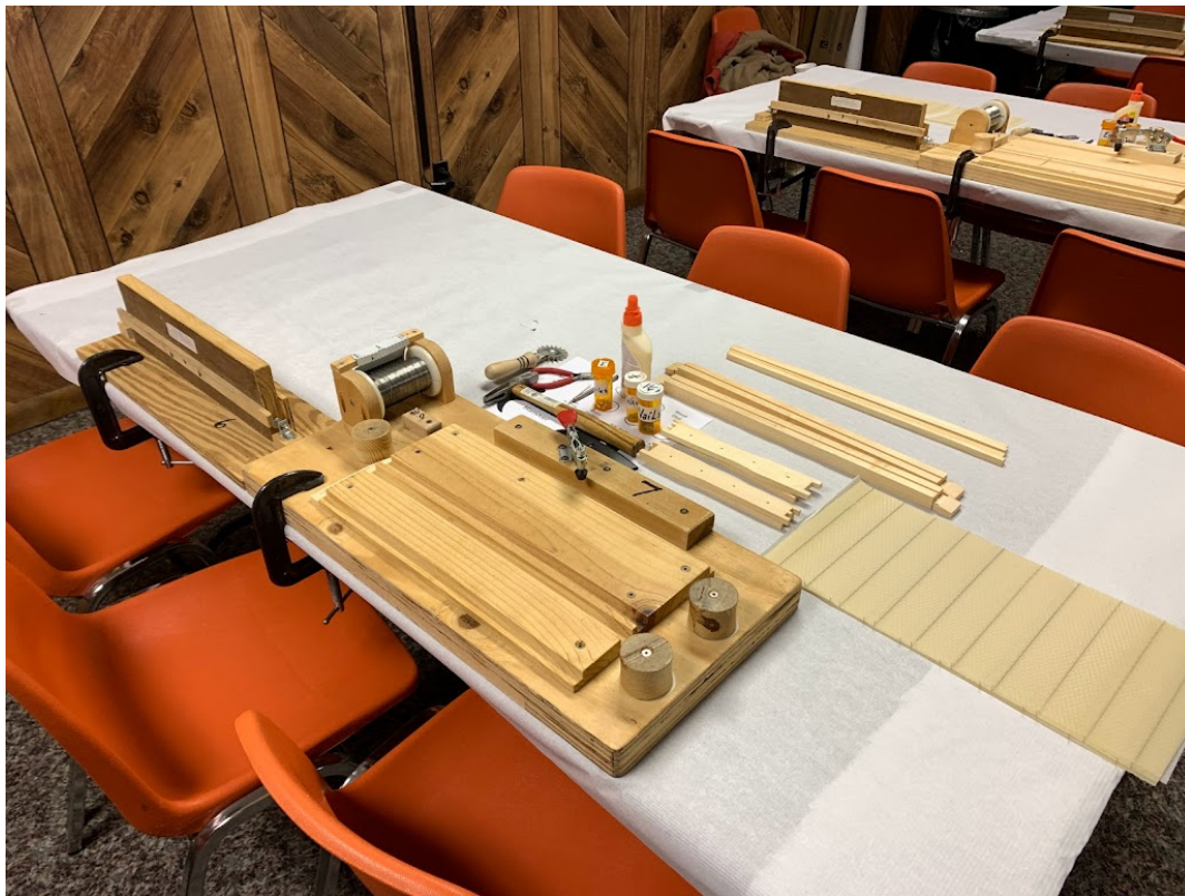
Jigs to build frame (left), and wiring jig
